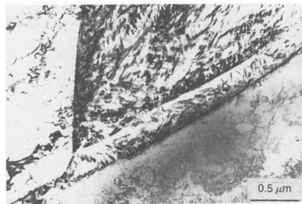
Figure 5 Martensite in steel B (60 sec at 575^\circ\text{C} ).
